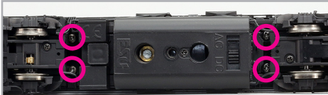
Figure 9: Seat of the housing screws
