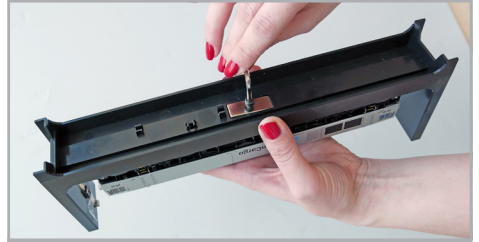
Figure 2: Unscrew the locomotive
