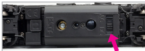
Figure 6: DC-AC switch on Position „DC“
